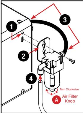
**A** Drain water from filter daily. Turn knob clockwise (from top view) to open. Drain. Turn knob counter-clockwise to close valve.
