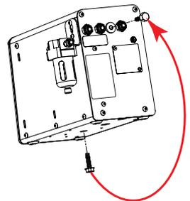
**FIG. 2 • Mounting Air Filter to Side**
